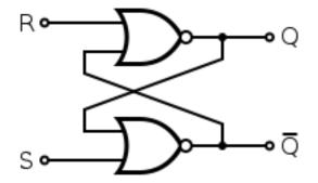
If the set input is 1 and the reset input is 0, gate 2 (bottom) will have an output of 1. But if either of the NOR inputs are 1, then the output has to be 0 regardless of the other input.
